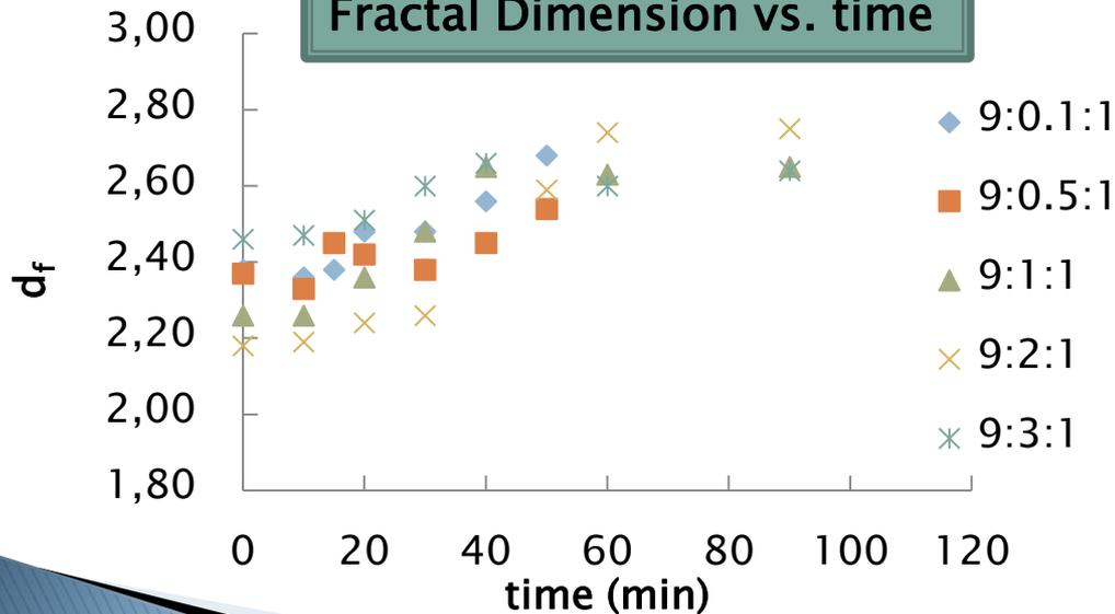
A time delay is observed between each release snapshot and the corresponding change of  $d_f$  which reflects the time of reorganization of the morphology of the nanostructure.
