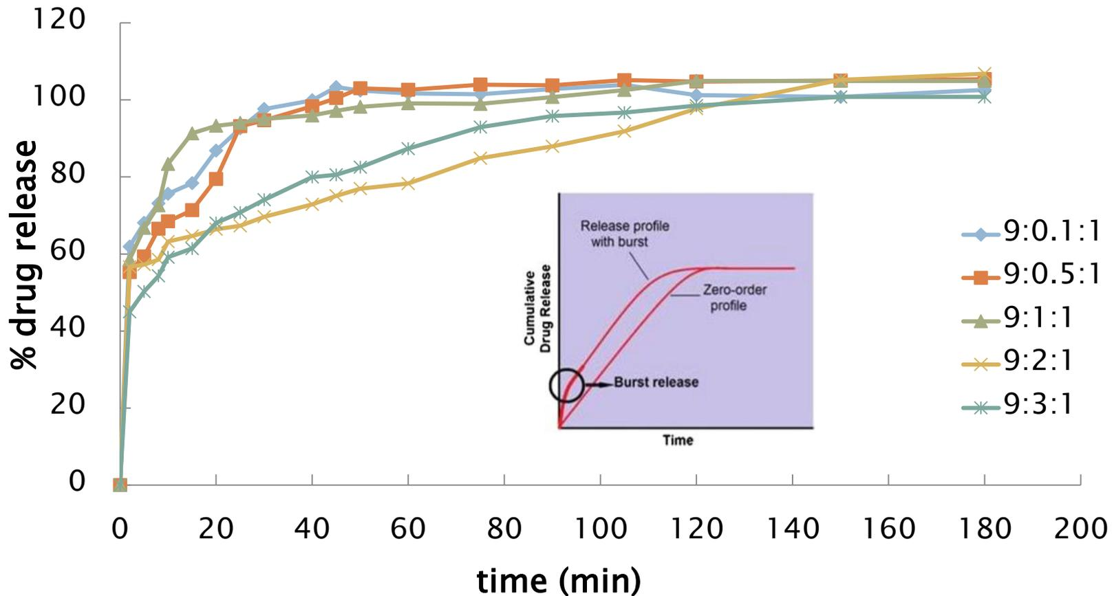
The *in vitro* release of the IND is faster from the polymer grafted liposomes with the lower ratio of gradient block copolymer. This phenomenology could serve as a guide factor for the preparation and development of formulations with the desired release profile, modulating the release rate of the IND via the ratio of the components, improving the release profile of the incorporating drug.
