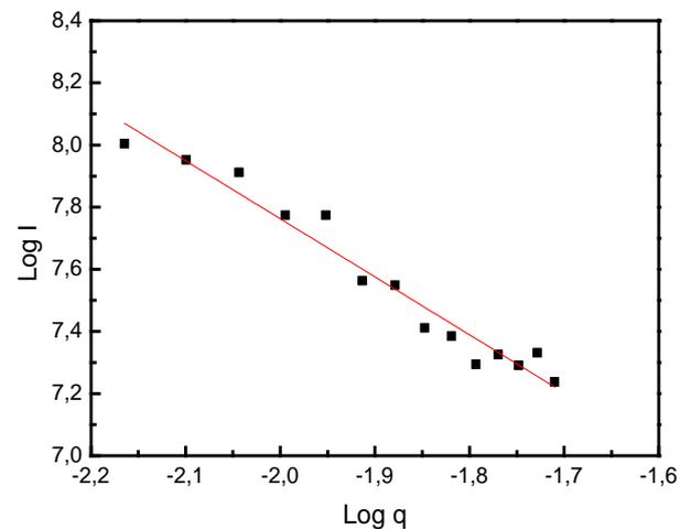
Log I vs. Log q plot for DPPC:PEO-b-PCL (9:1 molar ratio) chimeric nanoassemblies in HPLC-grade water.
